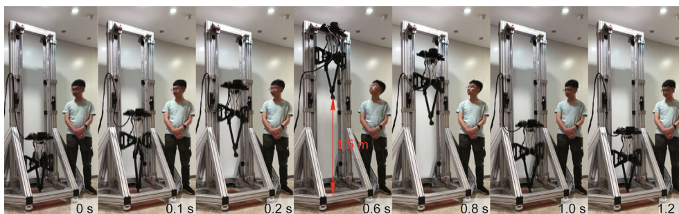
Fig. 11. Snapshots of jumping experiment with legged robot. The maximum jump height was 1.5 m.
