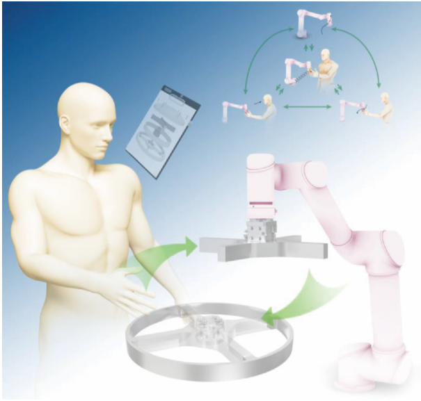
Fig. 1. HRC framework based on impedance control, where the human is the decision maker, the robot acts as the executor, and the assembly environment provides constraints.
