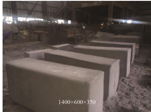
Fig. 4. NG-CT-50 ultrafine graphite blanks.
