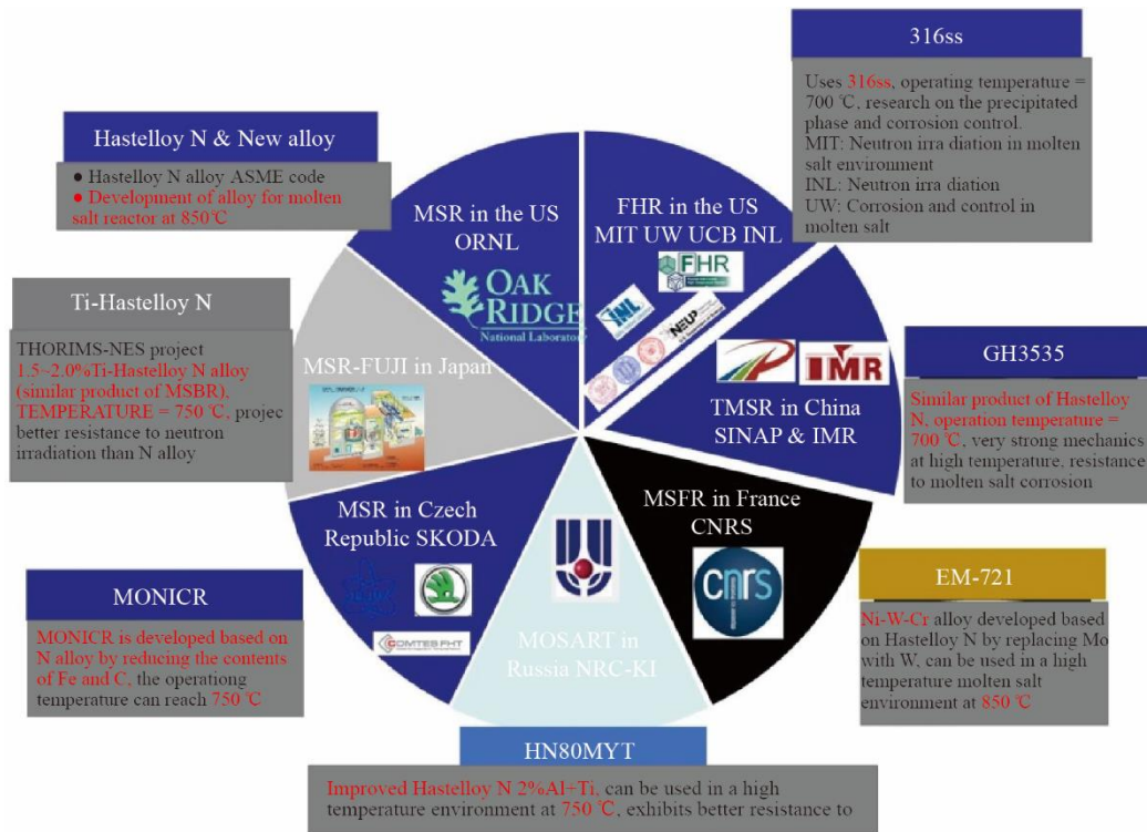
Fig. 1. Summary of research studies on the alloy structural material of molten salt reactors in China and abroad.
