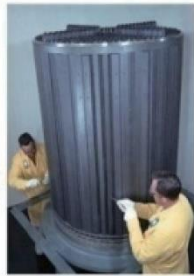
First generation nuclear graphite Representative products: CGB (MSRE), AGOT, PGA (early gas-cooled reactor)
