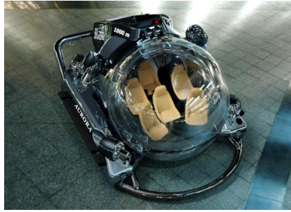
Fig. 7. Fully transparent window with extended fields-of-view.
