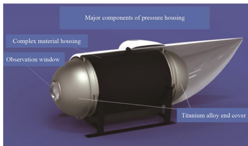
Fig. 6. Complex material pressure shell.
