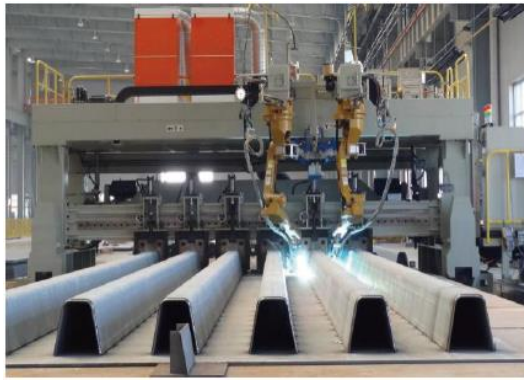
(a) Automatic assembly and positioning machine for U-shaped rib unit
