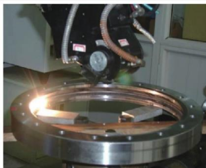
Fig. 3. Laser deep quenching of heavy-duty bearings.
