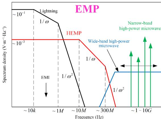
**Fig. 1.** Typical spectrum of different EMPs.
