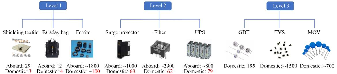
**Fig. 4.** Commercial products for EMP protection.
