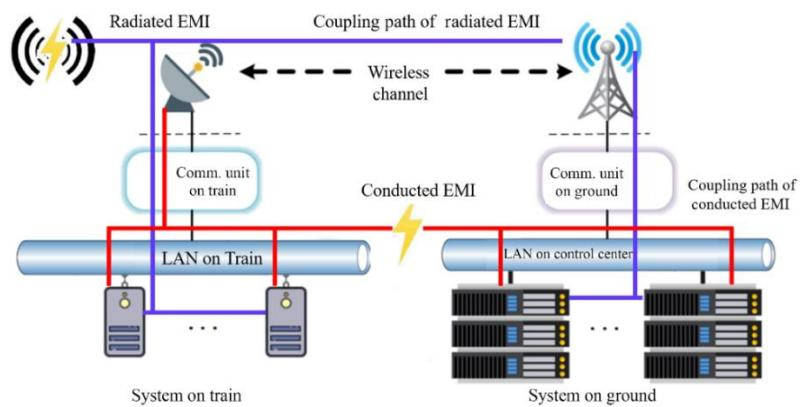
**Fig. 2.** EMI coupling paths in a typical high-speed railway control system.
