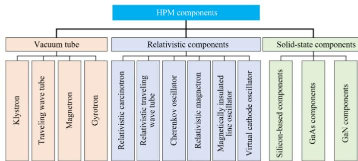
**Fig. 3.** Typical types of HPM components.
