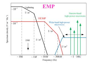
Fig. 1. Typical spectrum of different EMPs. Note: HEMP refers to high-altitude nuclear EMP; EMI refers to electromagnetic interference;
