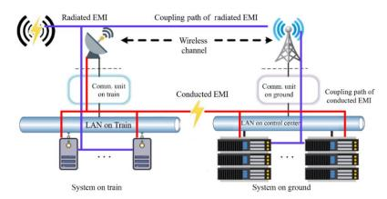
Fig. 2. EMI coupling paths in a typical high-speed railway control system. *Note:* LAN refers to local area network
