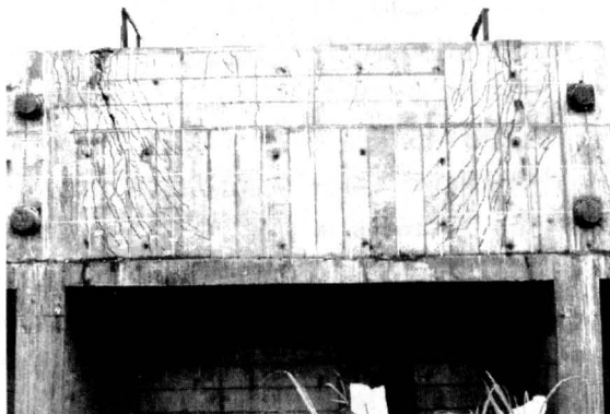
图 7 模型长边外立面裂缝分布 Fig.7 Cracking on long-side of the pylon model
