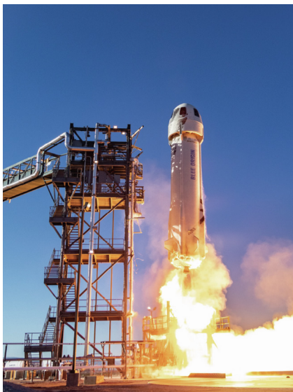
Fig. 3. Blue Origin's New Shepard capsule launches aboard its reusable booster rocket, carrying a payload of nine NASA experiments, on 23 January 2019. Note the large viewing windows on the capsule. Credit: courtesy of Blue Origin (public domain).
