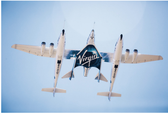
Fig. 1. Virgin Galactic's carrier aircraft VMS Eve shuttles the spaceplane VSS Unity on a test flight. Credit: courtesy of Virgin Galactic (public domain).
