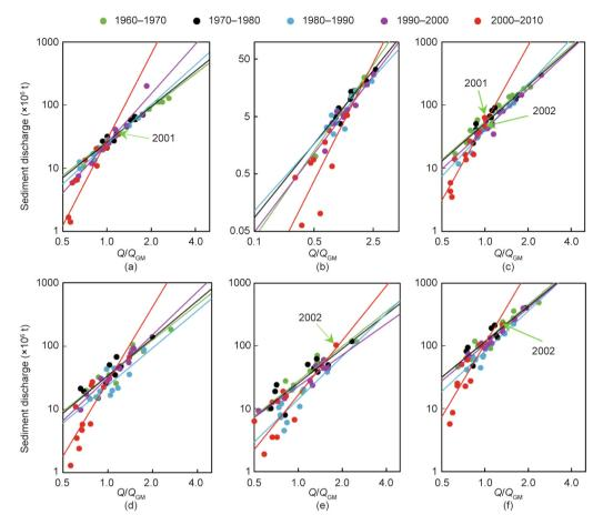
Fig. 5. Annual scale sediment rating curves at five stations: (a) Wuqi, (b) Zhidan, (c) Liujiahe, (d) Ganguyi, and (e) Yanchuan, and in (f) the entire study area during different time periods.
