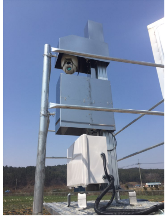
Fig. 2 Real-time onion disease monitoring system
