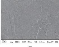
**Fig. 5.** Typical microstructure of IN718. (a) 3D view; (b) higher magnification showing column structure in XZ plane.
