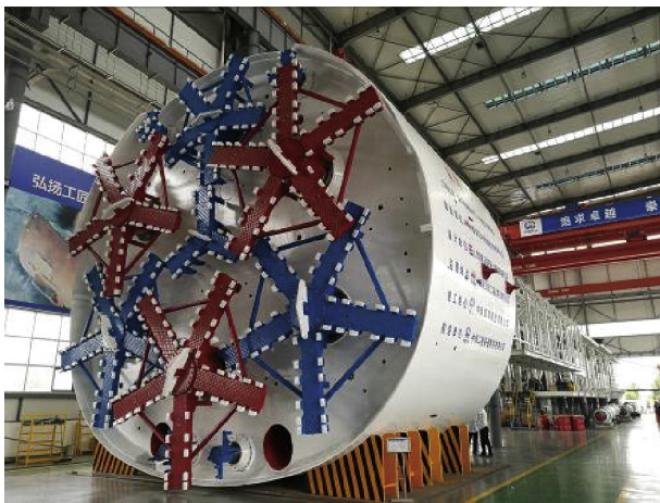
Fig. 3. The world's first horseshoe-shaped TBM.
