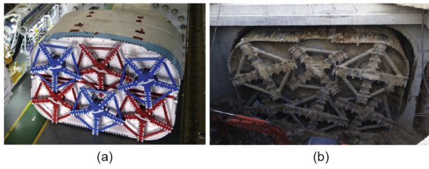
Fig. 9. (a) Super-large rectangular pipe-jacking machine; (b) front shield after breakthrough.
