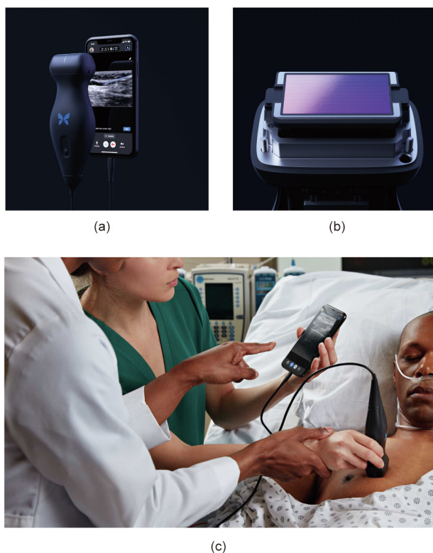
Fig. 2. (a) A wired handheld device, the Butterfly Network iQ+ ultrasound system is connected to a smartphone by a wire. (b) Within its head, the device contains an ultrasound-generating silicon chip comprising a two-dimensional array of 9000 micro-machined sensors (shown with the probe's upper casing removed). This technology allows the unit to emulate both a linear and curvilinear probe with a single head. (c) A physician uses the iQ+ on a patient. Credit: Butterfly Network, with permission.
