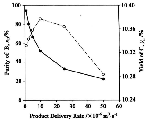
图 6 产品采出速率对产品纯度和收率的影响 Fig.6 Effects of delivering rate on the product purity and yield
