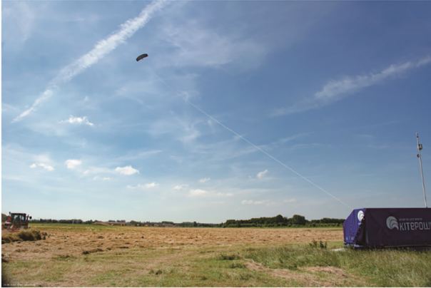
Fig. 2. A ground-gen AWE system flies its kite above an agricultural field in June 2018 at the former naval airbase Valkenburg in the Netherlands, now a European testing and training center for unmanned aerial technologies including AWE and drones [15]. To efficiently collect wind energy as it moves away from its base station (lower right), this autonomous, 25 m 2 kite maneuvers in cross-wind loops or figure 8s that transfer maximum force from the wind to pulling the kite's tether. As it unreels, the tether spins a generator that converts this wind-powered pull into electricity. Credit: Kitepower BV, with permission.
