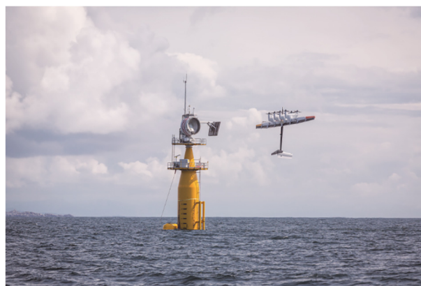
Fig. 1. The prototype, 600 kW energy kite made by Makani to autonomously harvest power from offshore winds hovers during flight tests near the coast of Norway in August 2019. The kite connects to its floating base-station by a tether attached to its 26 m wing that spools from the drum near the top of the structure. The kite lands and takes off from the tilted plate to the right of the drum which fits into a groove beneath its wing's bank of motor-generators. Credit: Makani Technologies, with permission.
