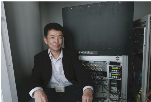
Fig. 1. Professor Hidetoshi Katori kneels next to one of the two transportable optical lattice atomic clocks—this one at the top of Tokyo's Skytree tower (see Fig. 2), the other at the bottom—which used the clocks' ability to measure the second to 18 decimal places in an experiment testing Albert Einstein's prediction of time dilation with the greatest precision ever for a ground-based clock [2]. Each of the transportable clocks, built by Katori and colleagues at the University of Tokyo, consists of three boxes with a total volume of roughly one cubic meter. Credit: Courtesy of Hidetoshi Katori.
