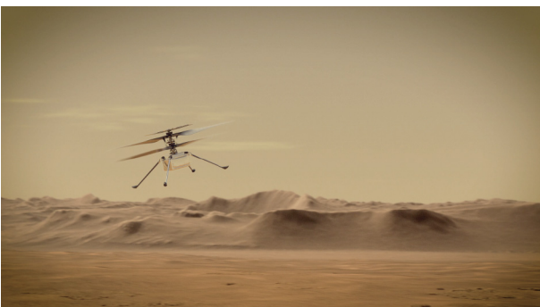
Fig. 2. The Perseverance rover can launch a miniature helicopter about 0.5 m tall and weighing 1.8 kg. If the "Ingenuity" helicopter succeeds in flying, as depicted in this artist's rendering, it will be the first craft to do so on another planet. To generate lift in Mars' thin atmosphere, Ingenuity's blades will spin at 2400 revolutions per minute, around five times faster than the average helicopter on Earth. NASA expects it to make five short test flights lasting about 90 s each. Credit: NASA/JPL-Caltech (public domain).
