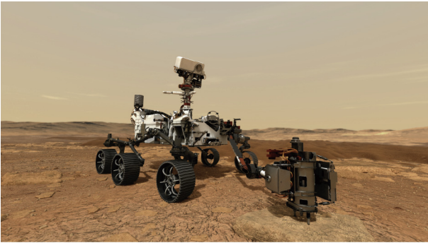
Fig. 1. An artist's rendering shows NASA's Perseverance rover drilling rock cores, which may contain evidence of past life, in Mars' Jezero Crater. The rover will collect and store about 30 rock and soil samples for a future mission to pick up and return to Earth. Credit: NASA/JPL-Caltech (public domain).
