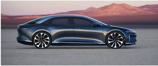
Fig. 1. The battery of Lucid Motor's Air model will power a range of more than 800 km on a single charge, thanks to design features that reduce air resistance and mechanical friction and upgrades in the efficiency of nearly every aspect of the electric drive chain. Credit: Lucid Motors (public domain).
