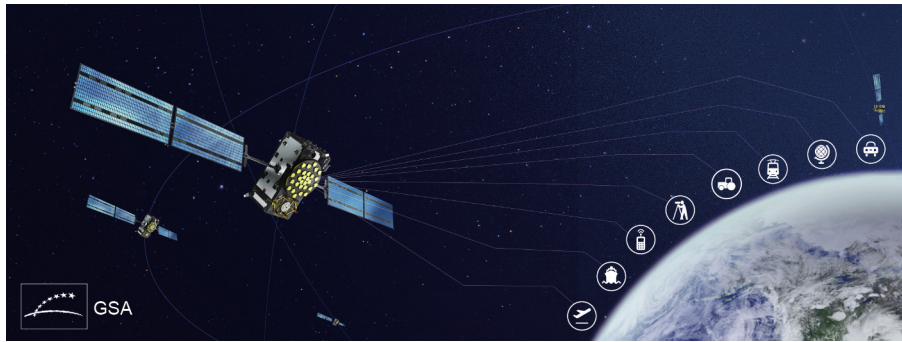
Fig. 2. An artist's illustration highlights one of the solar-powered spacecraft in the European Union's Galileo constellation of navigation satellites as it circles the planet in a medium-Earth orbit at an altitude of just over 23 200 km. The satellite's main antenna (disk studded with gold blocks at the front-center of the craft) continuously broadcasts timing and position radio signals to Earth, providing data used globally by billions of people, smartphones and other devices, and networks across a range of industries, services, and other fields, including aviation, surveying, agriculture, transportation, and others. Nearing completion, Galileo awaits additional launches in 2021–2022 to reach its full operational complement of 30 satellites, including six spares. GSA: European GNSS Agency. Credit: ©GSA, with permission.
