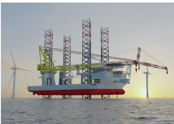
Fig. 3. An artist's illustration of the Voltaire jack-up vessel that is being manufactured by Belgium's Jan de Nul Group. In 2022, the vessel will be used to install the first commercial Haliade-X turbines, at Dogger Bank Wind Farm in the North Sea. Credit: Jan de Nul Group, with permission.
