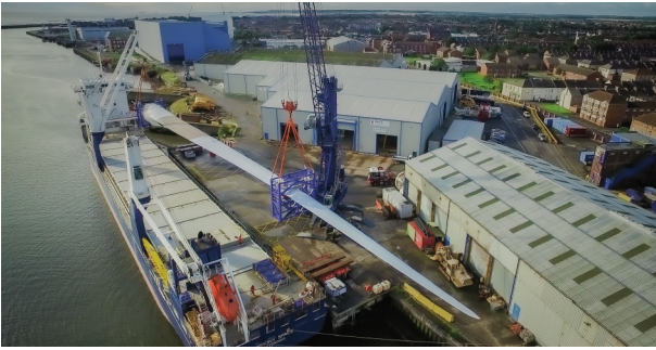
Fig. 4. A 107 m long Haliade-X blade arrives at the UK's Offshore Renewable Energy Catapult facility in Blyth to begin independent testing. Credit: Offshore Renewable Energy Catapult, with permission.
