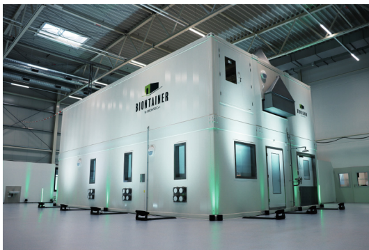
Fig. 1. BioNTech's modular factory for manufacturing the mRNA vaccine it developed with Pfizer consists of a drug substance module and a formulation module. Dubbed the BioNTainer, the factories are designed to produce up to 50 million doses a year at a cost far less expensive than building a traditional factory. Credit: BioNTech (public domain).
