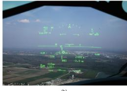
Fig. 2. (a) The radio altimeter is most important when planes are at low altitude, and particularly for landings in low-visibility conditions. (b) The head-up display in an aircraft cockpit projects key flight information such as altitude and air speed onto a screen in the pilot's line of sight. It is one of the systems that depends on the radio altimeter and could be disrupted by 5G interference. Credits: Vincent Albos (CC0); Joschiki (CC BY-SA 3.0).
