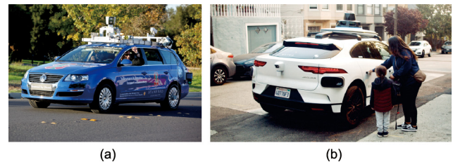
Fig. 1. (a) A prototype self-driving Volkswagen from Stanford University in Palo Alto, CA, USA and (b) a robot taxi from Waymo (Mountain View, CA, USA), Google's self-driving car spinoff company, feature large rooftop LiDAR units that help them sense and navigate their surroundings. Credit: (a) Flickr (CC BY 2.0); (b) Waymo (public domain).
