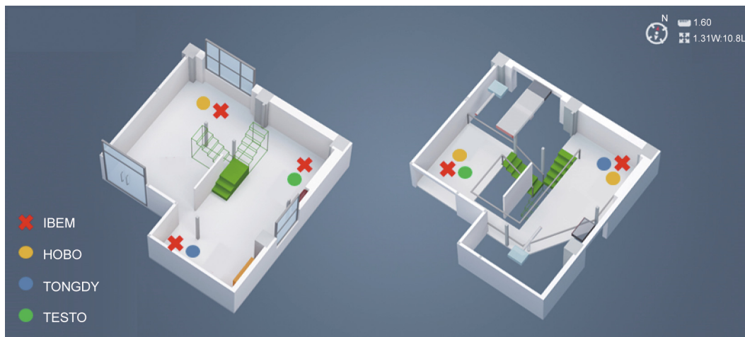
Fig. 5. Placement of IBEM and commercial devices for co-location testing.
