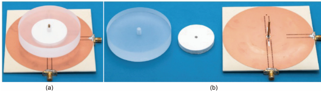
Fig. 11. Photos of the tri-band pattern-diversity DRA prototype. (a) Perspective view; (b) DR and feeding circuit.
