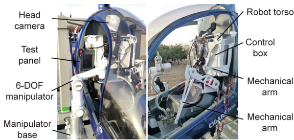
Fig. 17. Helicopter installation of the robot pilot.
