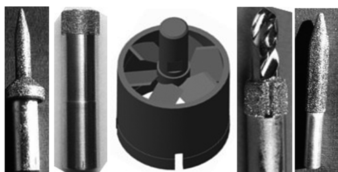
图8 系列金刚石磨料多刃工具 Fig.8 Diamond abrasive tools with multiple cutting edges
