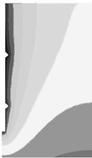
图 11 第四级荷载下单桩周围土体沉降图 Fig. 11 Settlement diagram of soil around single pile under the fourth grade load
