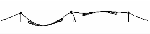
图4 60%施工状态一阶竖弯振型 Fig.4 The first vertical mode shape at the 60% construction stage
