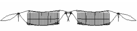
图5 60%施工状态一阶扭转振型 Fig.5 The first torsional mode shape at the 60% construction stage
