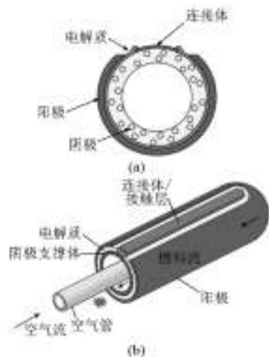
图5 阴极支撑管式SOFC单电池示意图 Fig.5 A schematic of single cathode-supported tubular SOFC
