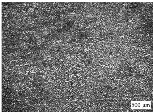
图12 隆起内侧的晶粒细化照片 Fig.12 Grain refinement inside the upheaval
