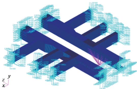
图10 车体局部结构的精细化仿真分析 Fig. 10 Accurate simulation analysis of car-body local structure
