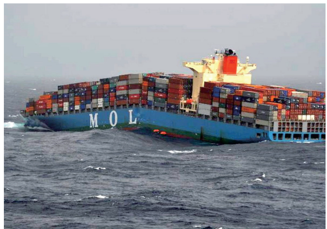
图 4. 因船体梁处承受过大的波浪应力而船体断裂的例子。(http://www.rina.org.uk/mol_comfort_accident.html, 12 February 2015)
