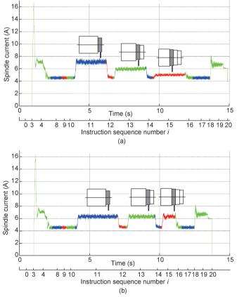
Figure 9. A comparison of the parameters of the three-step part (a) before and (b) after optimization.
