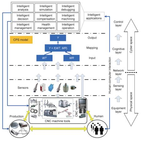
Figure 1. The CPS architecture of CNC machine tools with a CPS model.
