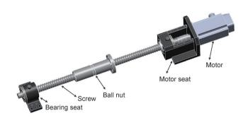
Figure 15. The feed axis mechanism of X axis.
