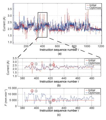
Figure 13. (a) The instruction-domain waveform of the spindle current; (b) a partially enlarged drawling of spindle current; (c) a partially enlarged drawing of feedrate.
