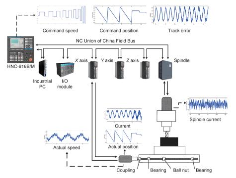
Figure 7. Big data acquirable inside a CNC machine tool.
