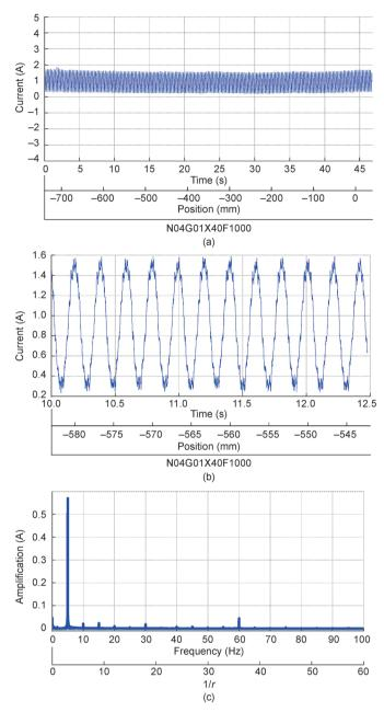
Figure 16. An analysis of the X axis current. (a) Diagram of the original current in the time domain; (b) a partial enlarged drawing; (c) the global amplitude spectrum.
