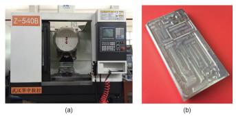
Figure 11. (a) The Z540-B drilling and tapping center; (b) the test part.
