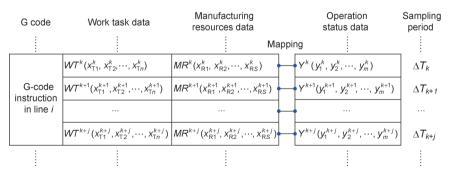
Figure 4. The mapping of work task data, manufacturing resources data, and operation status data of a CNC machine tool.
