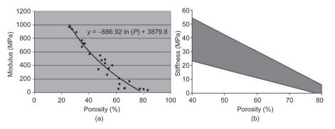
Figure 5. Scaffold porosity and mechanical property. (a) Relationship between porosity and modulus in FDM scaffolds; (b) the feasible porosity and compressive stiffness range (gray band) in SLS-made PCL scaffolds.
