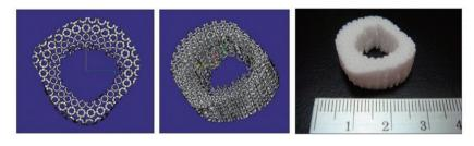
Figure 2. Virtual and physical prototypes of the functionally graded porous scaffold of a femur bone segment.
