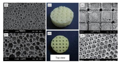
Figure 6. Highly and uniformly porous interconnected network via the combination of indirect 3D printing and foaming processes
