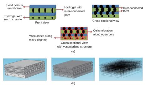
Figure 3. A proposed hybrid scaffold design for vascularization.
