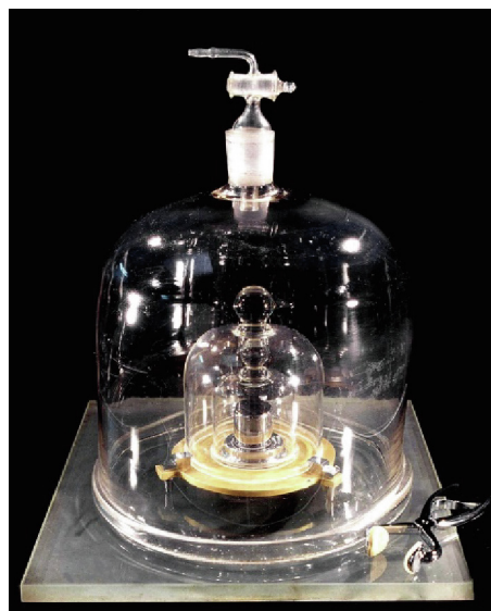
Fig. 1. Since 1889, a squat cylinder of platinum alloy known as Le Grand K has been the global standard for the mass of the kilogram. As it has since it was forged, Le Grand K sits under three glass bell jars in a vault outside Paris. Credit: BIPM.
