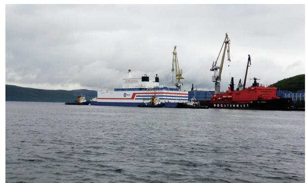
Fig. 1. On 23 August 2019, the first floating nuclear power station began its 4700 km journey from Murmansk in Russia to the port of Pevek, on the Eastern Siberia Sea, where it will be used to produce electricity for the region of Chukotka. The ship, capable of producing energy for a city of 100 000 inhabitants, will become the most northern nuclear facility in the world. The Akademik Lomonosov was built by the Baltic Shipyard in St. Petersburg and is owned by the Russian company Rosatom. Credit: Elena Dider, Wikimedia Commons (CC BY-SA 4.0).
