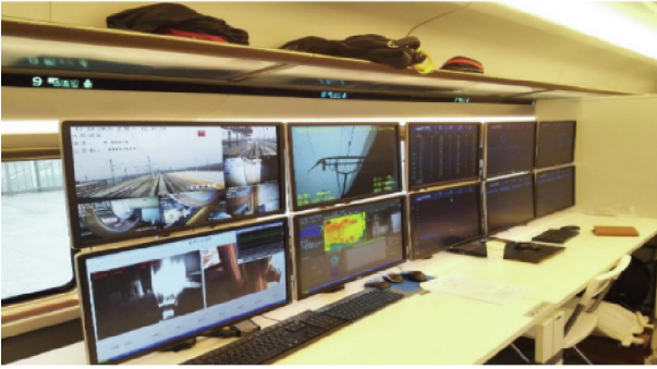
Fig. 11. The Fuxing EMU test-monitoring system.
