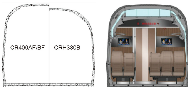
Fig. 10. Carbody cross-section of the Fuxing EMU.
