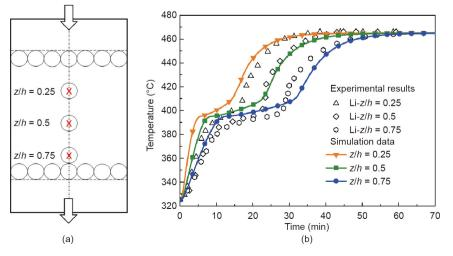
Fig. 5. (a) Position illustrations of thermocouples; (b) comparison of calculation results with experimental data.
