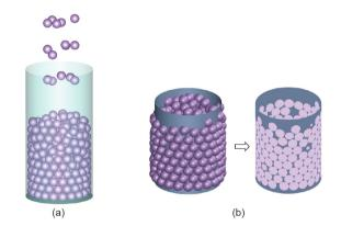
**Fig 1.** Schematic diagrams of (a) packing process of sphere and (b) generation of sub-surfaces along the radial direction.
