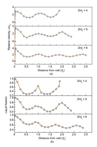
**Fig. 12.** Radial distributions of the packed bed LHS systems with different diameter ratios. (a) Relative velocity; (b) liquid fraction when *t* = 1200 s.
