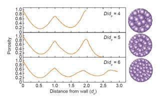
Fig. 11. Radial porosity distributions of the packed bed models with different diameter ratios.
