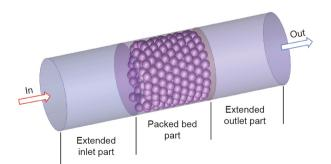
Fig. 3. Schematic diagram of 3D packed bed LHS system.
