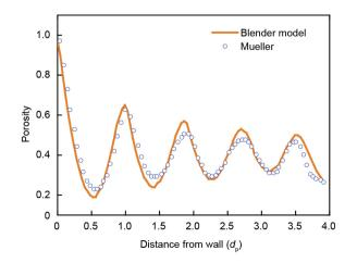
Fig 2. Comparison of radial porosity distributions when diameter ratio is 7.99.
