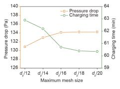
Fig. 4. Independence verification of mesh size.
