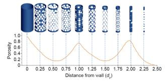
Fig. 6. Radial porosity distribution and sub-surfaces along the radial direction.
