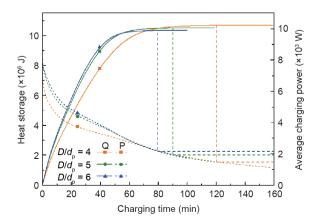
**Fig. 13.** Heat storage and the average charging power of the packed bed LHS systems with different diameter ratios.
