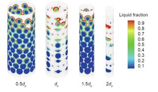
**Fig. 10.** Liquid fractions of PCMs on the radial sub-surfaces when t = 600 s.
