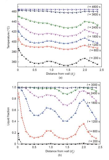
Fig. 9. Radial distributions of PCMs at different time. (a) Temperature; (b) liquid fraction.
