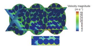
Fig. 8. Flow velocity distribution inside the packed bed.
