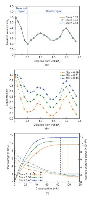
**Fig. 15.** Flow and thermal properties in the packed bed LHS systems with different Stefan numbers. (a) Radial relative velocity distribution; (b) radial liquid fraction distribution when t = 1200 s; (c) heat storage and the average charging power.
