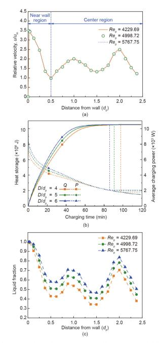
**Fig. 14.** Flow and thermal properties in the packed bed LHS systems with different Reynolds numbers. (a) Radial relative velocity distribution; (b) heat storage and the average charging power; (c) radial liquid fraction distribution when t = 1200 s.
