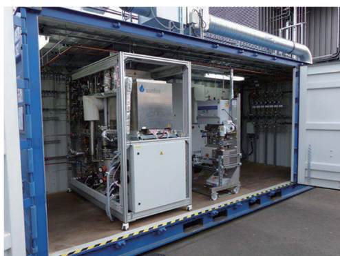
Fig. 13. A co-electrolysis system demonstration developed by Sunfire GmbH. Reproduced from Ref. [99] with permission.
