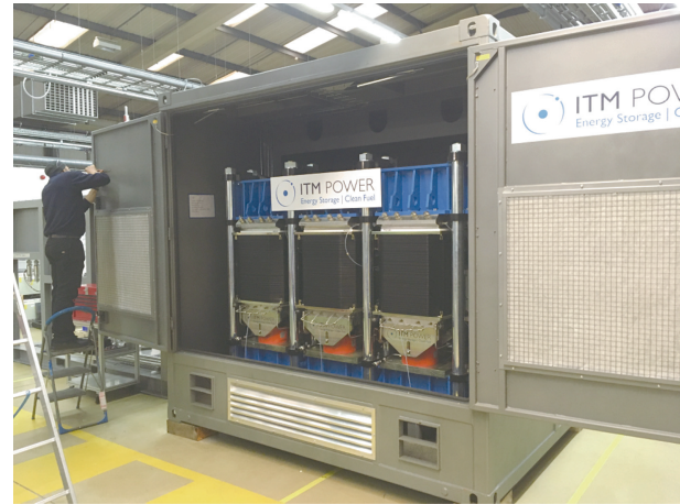
Fig. 3. Built in 2021 by ITM Power PLC at its factory in Sheffield, UK, this electrolyzer uses renewable energy to separate tap water into green hydrogen and oxygen gases. Credit: Wikimedia (CC BY-SA 4.0).
