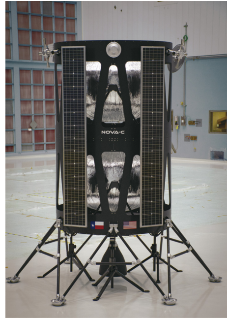
Fig. 2. The NOVA-C lander from Intuitive Machines is 3 m tall, 2 m in diameter, and can tote 100 kg of cargo. The craft will carry the Lunar Vertex mission, along with three other government space agency and commercial payloads, to the Moon's surface in 2024. The same model of lander is also booked for two previous missions scheduled to touch down near the Moon's south pole in late 2023. Credit: NASA (CC BY 2.0).
