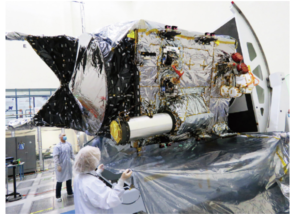
Fig. 2. The DSOC laser transceiver, encased in its tubelike sunshade protruding from the side of the Psyche spacecraft, set a record in 2023 for the longest optical data transmission at 1.6 \times 10^7 km. Credit: NASA/JPL-Caltech (public domain).
