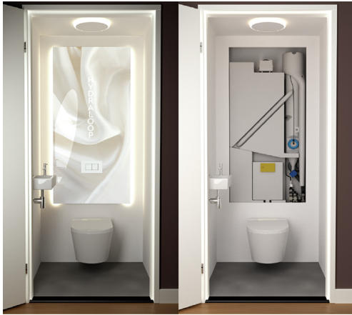
Fig. 2. Packed behind the Hydraloop's concealing faceplate (left) is a system (right) capable of recycling 0.2 m 3 of water per day. The system, which costs 1995 USD, removes dirt, soap, and other pollution from greywater without the use of filters, membranes, or chemicals. Flushed water is piped up to the top of the treatment tank on the right, then travels down to be treated with six different technologies: sedimentation, floatation, dissolved air floatation, foam fractionation, an aerobic bioreactor, and disinfection of the cleaned water with powerful ultraviolet light. Waste is piped into the sewer. A pump under the tank redistributes the treated water for reuse, including in toilets and washing machines. Credit: Hydraloop Systems (public domain).
