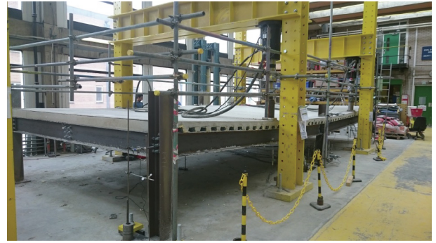
Fig. 22. Deflection of the edge beam due to missing support to the central column.
