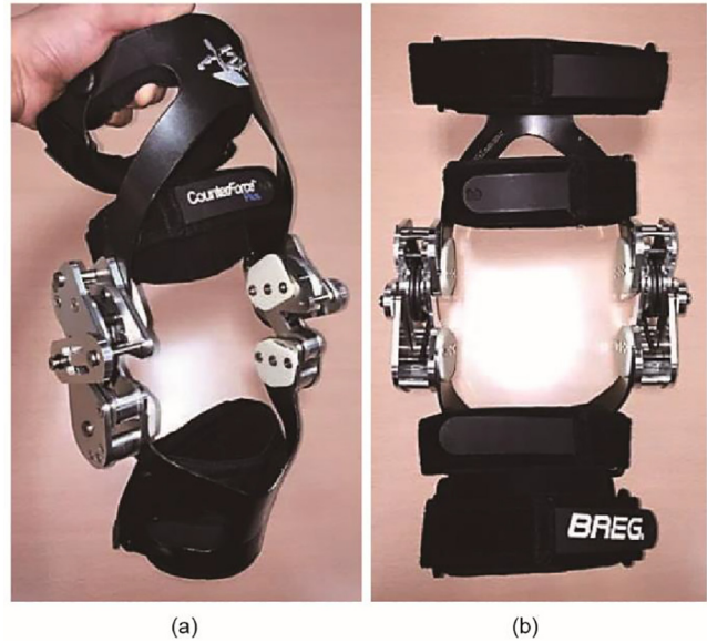
Fig. 7. Unpowered knee exoskeleton prototype modified from the Breg X2K. (a) Side view; (b) front view.
