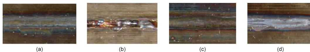
Fig. 6. Definition of four kinds of welding status. (a) Sound well weld; (b) blowout; (c) humping; (d) undercutting.
